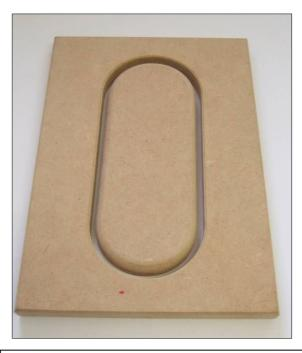
Female former is larger than male former by thickness of casing material
