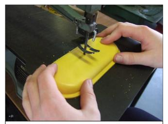
Cut the formed casing in half and draw file to finish
