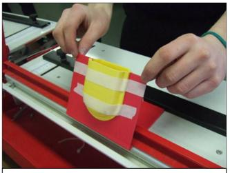
Bend the support bracket using a strip heater
