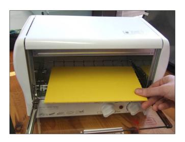
A piece of 120x200x3mm Foamex is placed in pre heated oven
