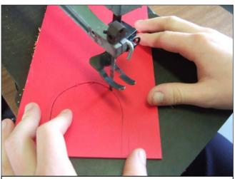
Cut the profile approx. 10mm smaller than the casing
