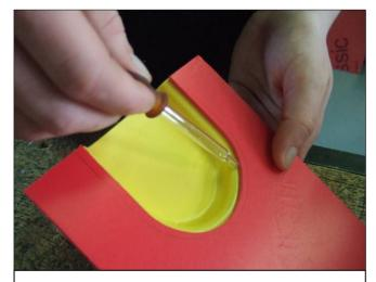
Affix both materials using tensol solvent/cement or a glue gun
