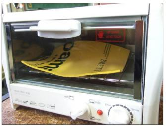
The material is heated for approximately 30 secs. At 140°C
