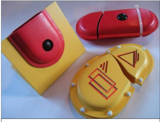
A variety of solutions can be achieved using the Plug and Yoke method of Press Forming
