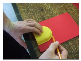
Mark the casing profile on a different colour piece of Foamex
